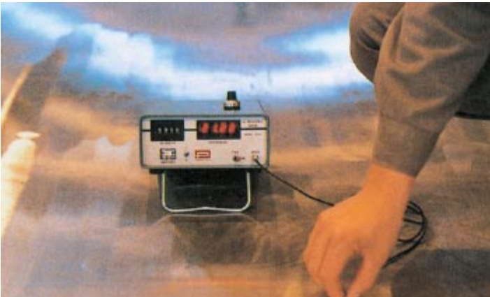
Plate thickness measurement
