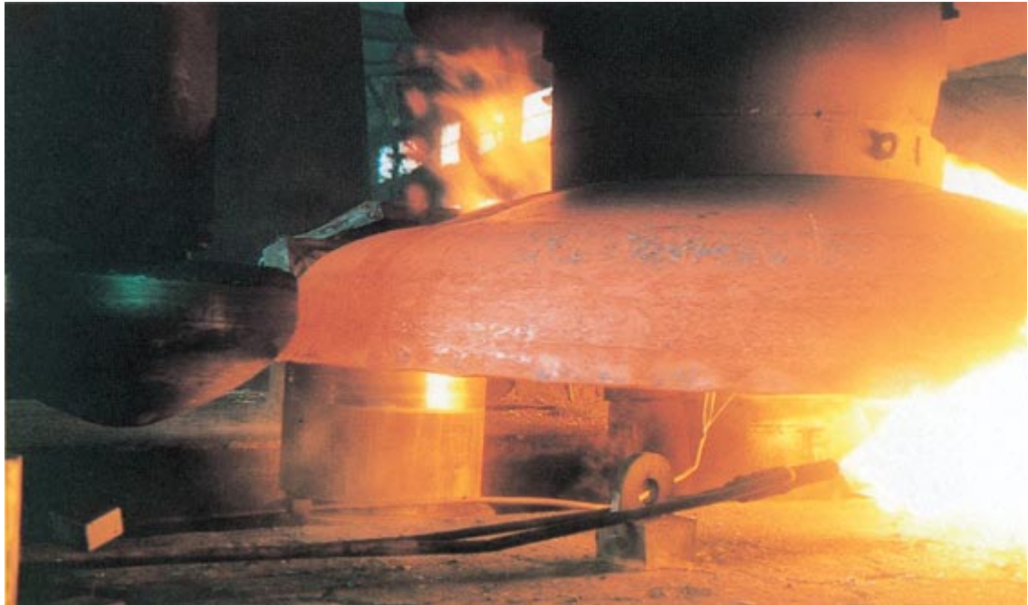
Shaping of head in progress
