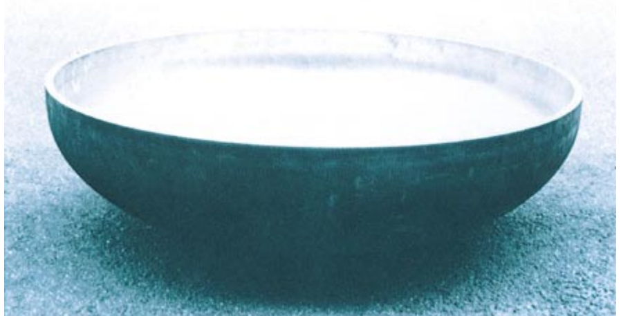
Appearance after shaping of a head plate
